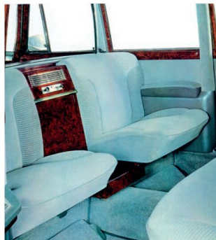
LEFT In Pullmans the two extra seats could be front- or, as shown here, rear-facing.
