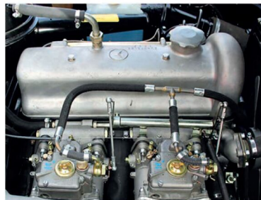
... which is why twin Weber 40 DCOEs are a common W121 engine modification.
