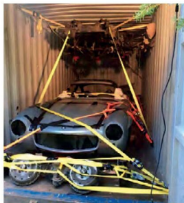
Engine and transmission out, and the chassis hung from the container's roof.
