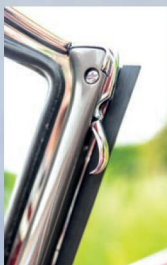
The canvas hood attaches to the front screen with easily operated catches.
