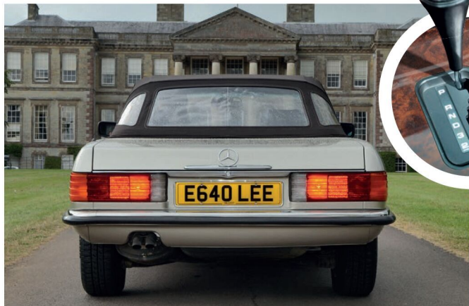
ABOVE RIGHT INSET Four-speed autobox works smoothly, but check it doesn't clunk into reverse.
