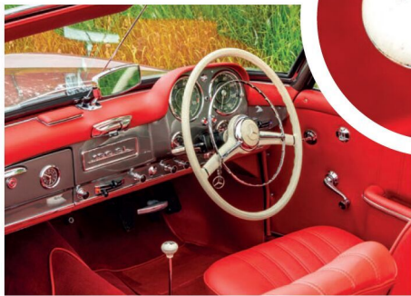
ABOVE INSET All 190SL used a four-speed manual gearbox, with a quite vague shift.
