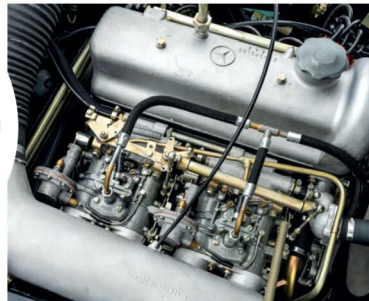
Worn original Solex carburettors cause poor engine running, and perplex owners...
